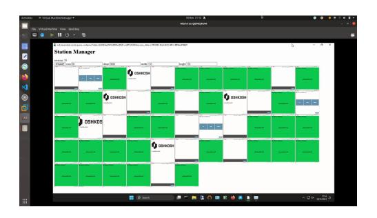
Station Manager is a tool that manages multiple test applications running simultaneously and independently, each connected to different testing devices or vehicles.
