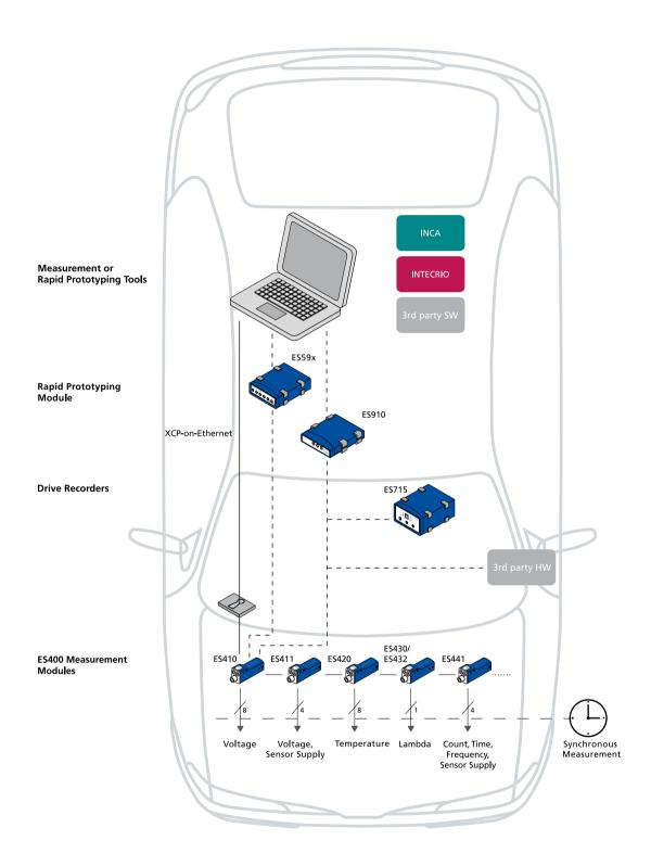
Figure 3: ES400 modules mounted in the engine compartment are connected through a "keyhole" to the PC in the vehicle interior. As an alternative to the PC hosting the INCA measurement, INTECRIO rapid prototyping, or third party application, the modules can deliver their data to the ES910 Rapid Prototyping Module or an ES720 Drive Recorder. XCP-on-Ethernet facilitates the integration with software tools or hardware devices from third-party manufacturers.
